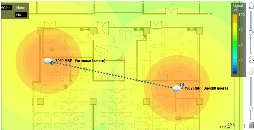
Figure 222. Dotted lines indicate that these APs are part of the wireless mesh network
